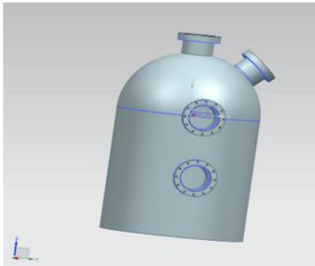
**Figure 5.** The NX model created to include second valve
