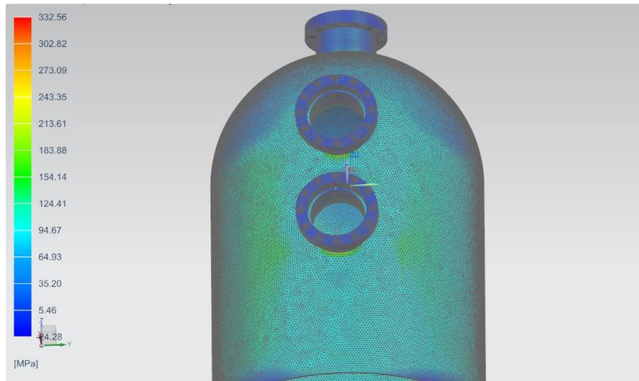
**Figure 6.** FEA result with valves in the cylindrical section 170 mm apart
