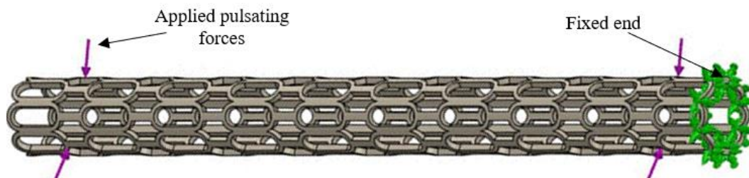
Figure 3. Stent model setup for non-linear dynamic analysis showing a location where pulsating forces applied
