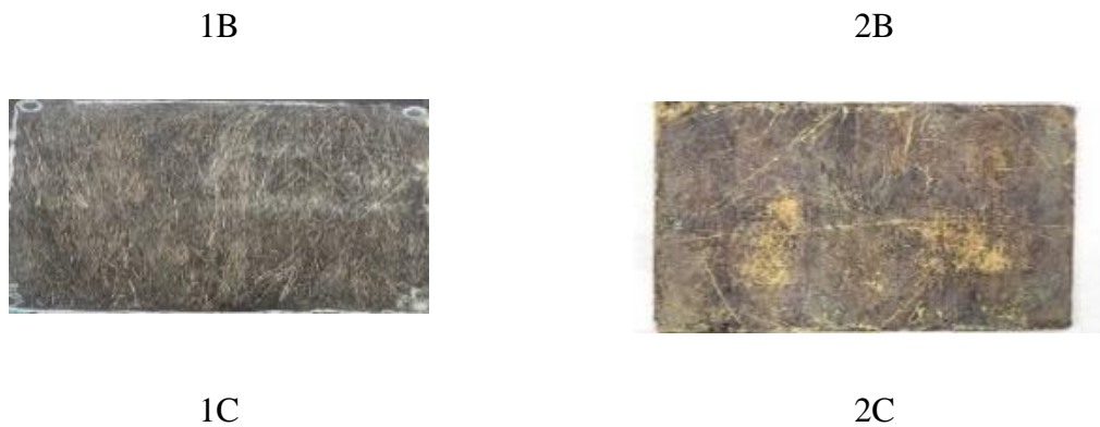
Figure 5. Specimen of the date palm fibre polymer composites
