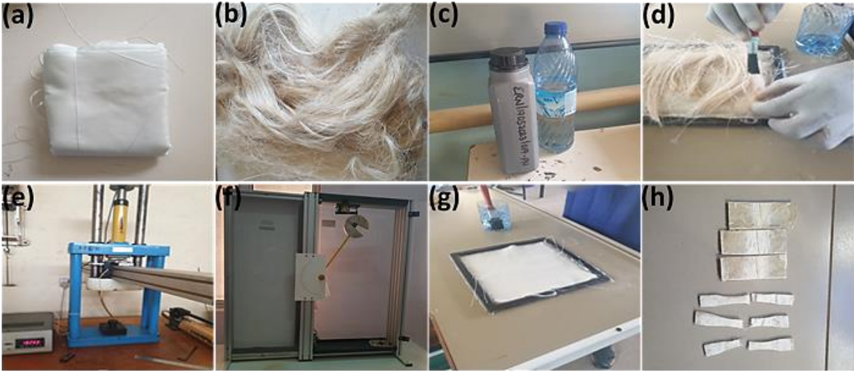
Figure 1. The equipment, machines, and processes for the experiment. (a) glass fibre, (b) sisal fibre, (c) epoxy resin and hardener, (d) hand-layup process of sample 2, (e) universal testing machine, (f) Charpy impact testing machine, (g) hand lay-up process of glass fibre 30wt% + sisal fibre 10wt%, and (h) tensile test specimen
