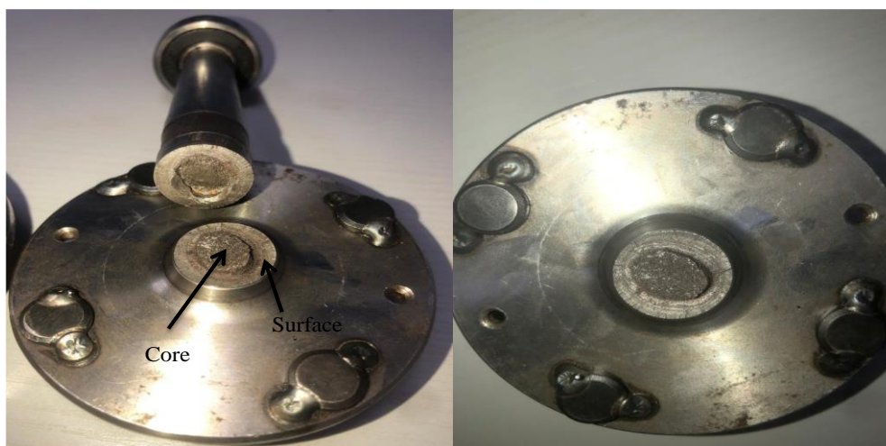
Figure 2. Fractured surface of a failed tricycle front wheel axle
