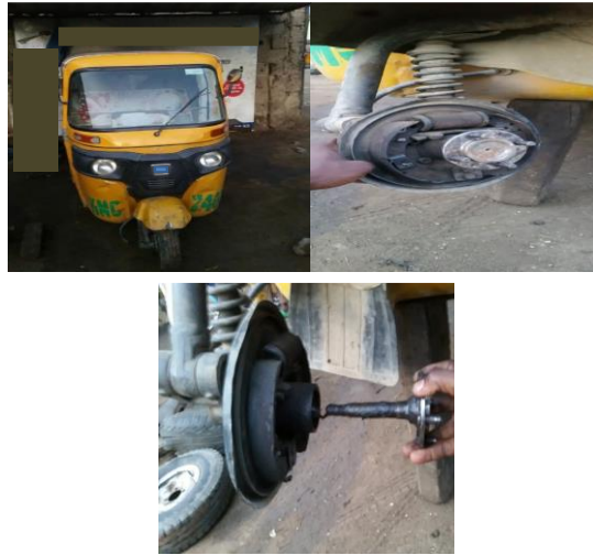
Figure 1. Tricycle vehicle and position of front wheel axle
