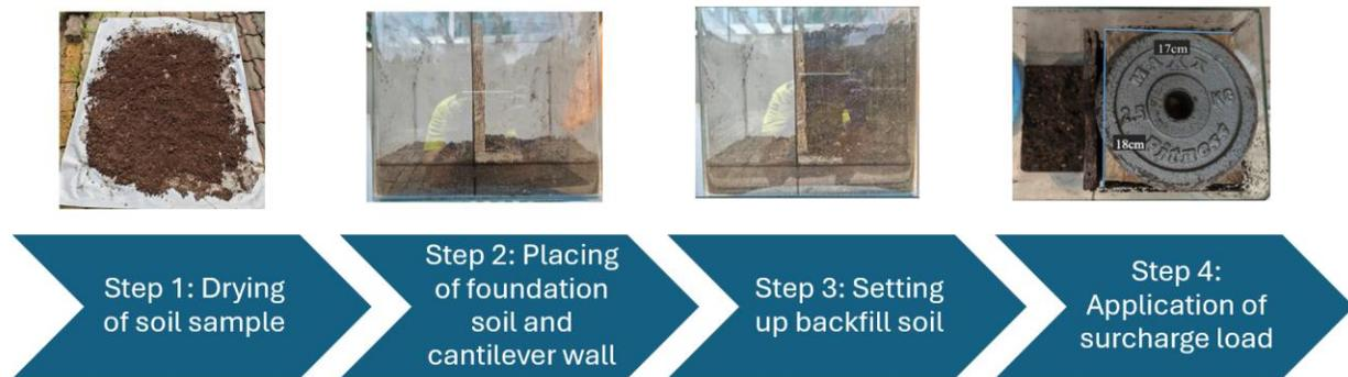
**Figure 3.** Experimental setup
